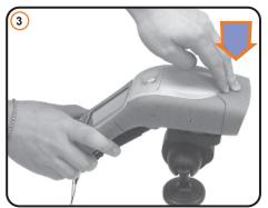
Press the front of the IKE down until the locking lever clicks into position.
