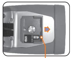
The tripod direction indicator arrow must point towards the front of the IKE.
