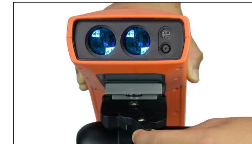
Hold the lever outwards and clip the tripod plate on the back of the IKE device to the tripod.
