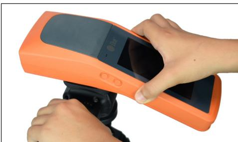
To adjust the position of the IKE device, squeeze the main lever and move to adjust. The lever can move in all directions.
