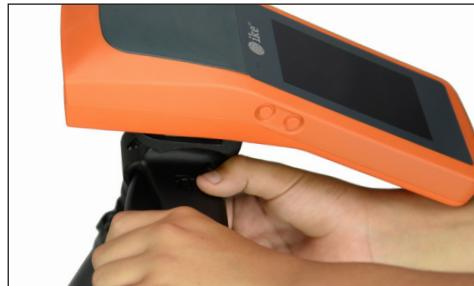
For span and pole height measuring, you can further tighten the movement of the lever so that the ball joint remains locked yet the pitch mechanism is still moveable. To do this, while pressing the main lever with one hand, use your other hand to turn the friction dial and adjust the tension. Test the tension of the movement between adjustments.
